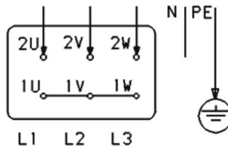
3. 3-phase dual-speed motors (double-winding), for example  $2p=6/4, 8/6$ :
