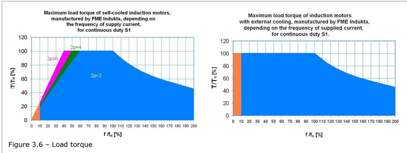
Figure 3.6 – Load torque
