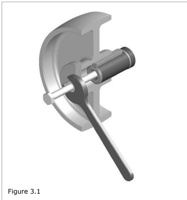
If necessary, heat up the coupling hub or the pulley /belt, geared/ to about 80°C.
