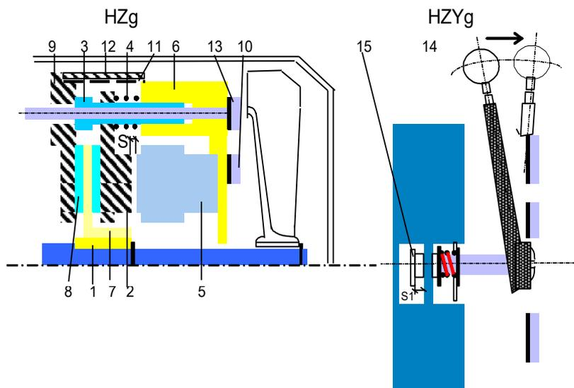
Alternating current fed to the electromagnet's winding (5) causes the  $S = 0$  armature to be shifted, eliminating the pressure of the springs on the armature, releasing the brake. In case of brakes with a lever (14) is it possible to manually release the brake by moving the lever; releasing the pressure causes it to automatically return to the starting position and repeated braking.
