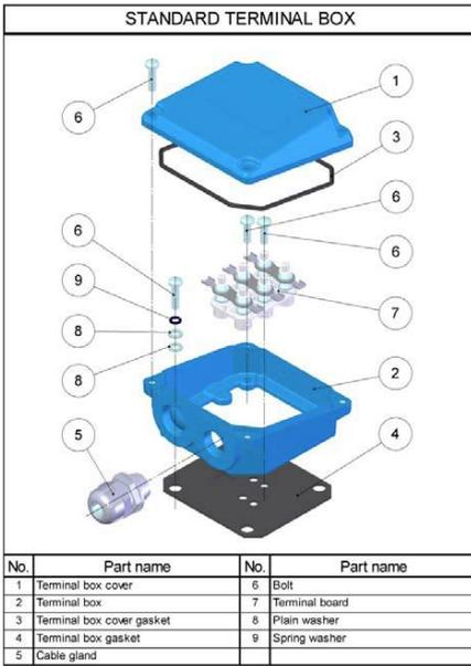
Disassembly of the motor's terminal box is done in accordance with the below drawing. Depending on the type of motor, following terminal box settings are available:
