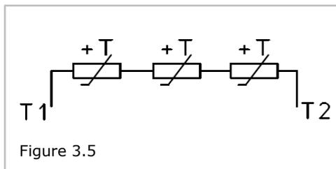
Sensor outlets should not be connected directly to the contactor's terminals. They should be connected to the resistance relay's terminals.
