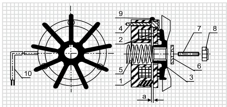
Switching off the electromagnet (1) causes the armature to be moved (2) through the springs until the torque is created and the brake lining is pressed against the ventilator. The brake is immobilized (halted).
