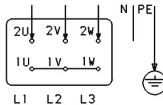
5. 3-phase dual-speed motors (nine terminals), for example 2p=4/2, 8/4:
