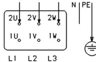
4. 3-phase dual-speed ventilator motor (single-winding), for example  $2p=4/2W, 8/4W$  – motor marking ending in „W“:
