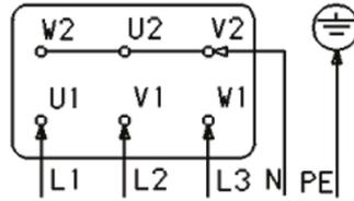
2. 3-phase dual-speed general use motors (single-winding), for example,  $2p=4/2, 8/4$ :
